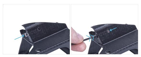
• Insert the M3nS nut into the External PSU bracket. Using the Allen key, push the nut all the way into the printed part and align the nut with the hole in the part.
