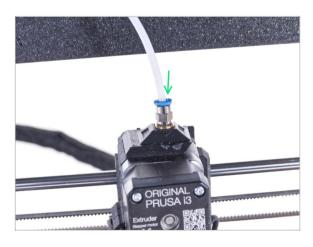
Insert the free end of the PTFE tube to the Fitting QSM-M5 on the extruder. Insert it all the way down.
