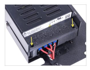
Mount the PSU cover back on the PSU using two M3x10 screws.
