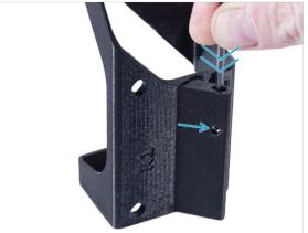
Insert the M3nS nut into the External-PSU-bracket-XP. Using the Allen key, push
