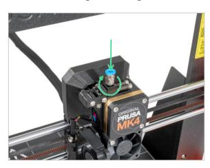
Insert and screw the Fitting QSM-M5 directly into the threaded filament hole in the extruder.
