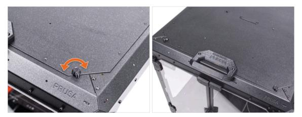
• Close the lid and turn both Lid-lock. If the locks turn stiffly over the lid, slightly loosen the screws on the bottom of the lock (inside the enclosure).
