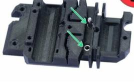
**⚠ For the following nut insertion USE A SCREW. THAT'S AN ORDER!!!** Seriously, use a screw to pull the nuts in, both have to be properly seated in the X-carriage.
