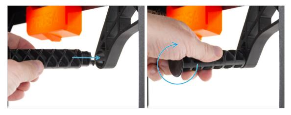
Insert the side arm into the Spool-holder-r and turn counter-clockwise to lock it.
