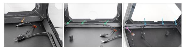
• Push the PSU cable through the circle hole in the rear of the Enclosure.
