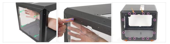
• Peel off the protective layers from both sides of the MINI Side panel.
