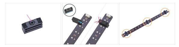
Insert the M3n nut into each LED Stick Bracket.
