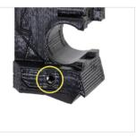
Always check the correct position of the M3nS nuts in the printed parts immediately after insertion. Improperly inserted nuts will not allow proper assembly of parts.
