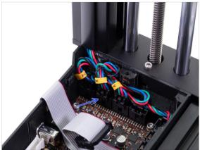
Connect the X-axis motor cable to the Buddy control board. Use the second slot from the left.
