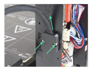
Attach the heatbed-cable-holder to the xBuddy box. The cable bundle must be pointing up. Secure it by tightening both M3x6 screws firmly.
