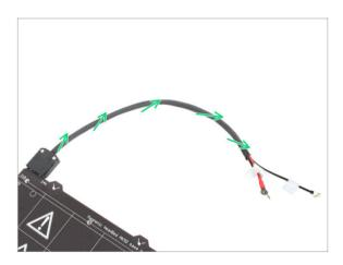
Finish wrapping the cable bundle in the textile sleeve. And twist the sleeve, **not the cables**.
