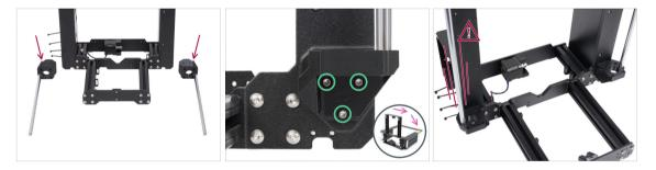
WARNING: Printed parts aren't the same! There are left and right pieces. See the protrusion (tooth) on each part. For the right side of the frame, there is a protrusion on the right side of the plastic part and vice versa.
