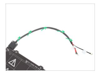
Finish wrapping the cable bundle in the textile sleeve. And twist the sleeve, not the cables.
