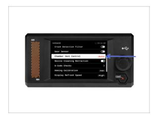
To enable automatic opening of the top grille, go to Settings -> Hardware -> Chamber Vent Control and set it to Auto.
