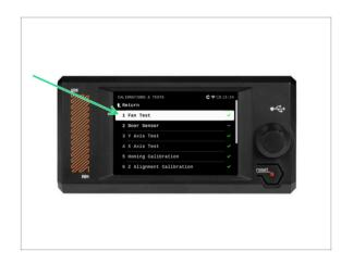
After finishing the upgrade, we recommend visiting the menu Control -> Calibrations & Tests and run the Selftest from the start.
